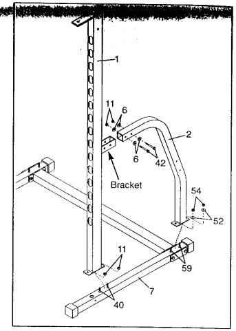
Slide the remaining Brace (2) onto the bracket on the other Upright (1). Attach the Brace to the Upright with two M10 x 65mm Bolts (42), four M10 Washers (6), and two M10 Nylon Locknuts (11). Do not tighten the Nylon Locknuts yet.
